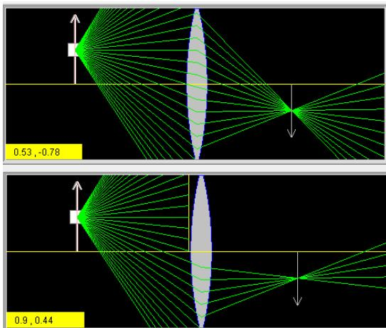
Exploration 35.1" in *Physlet Physics*. The box on the arrow (source) represents the diverging rays from that point on the arrow and it can be moved up and down to show how the image is formed (left). In the second part of the exercise, a screen can be added (right).
