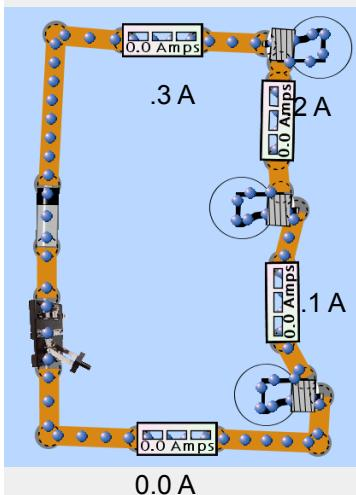
Figure 2 Circuit for what if anything is wrong task on electric current in a series circuit.
