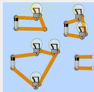
Figure 1. Four different “circuits” used for ranking task on terminal voltage of battery
